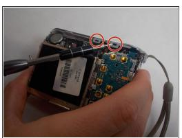
Release all clips and latches keeping the casing in place using a spudger, opening tool, or screwdriver.
