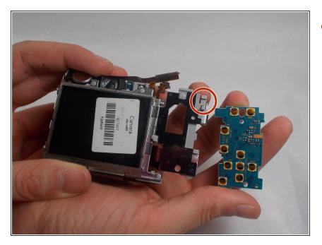
Unlatch the clip and lift the motherboard upwards and away from the camera.
