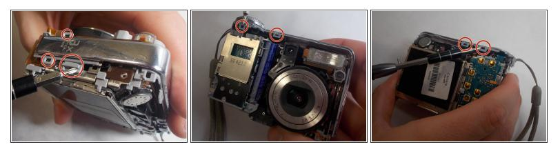
Release all clips and latches keeping the casing in place using a spudger, opening tool, or screwdriver.
