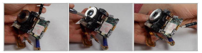
• Disconnect the three pictured ribbon cables using a spudger or screwdriver.
