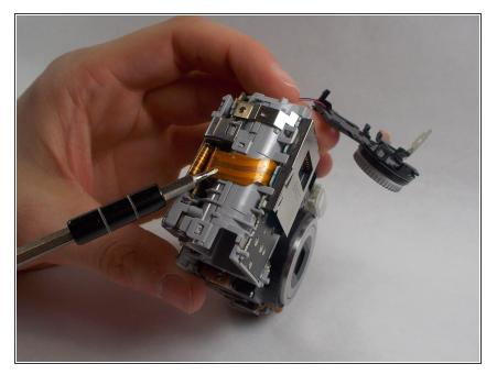
Disconnect the remaining ribbon cable on the side of the camera using a spudger or screwdriver.
