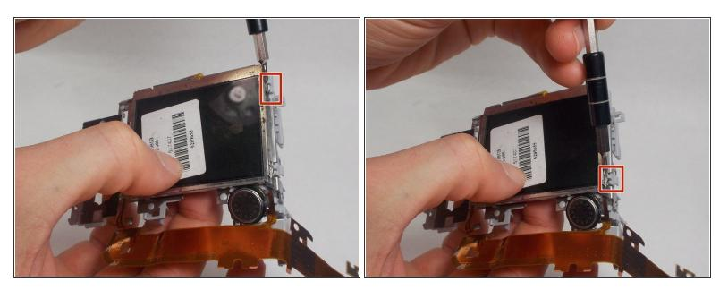
• Unlatch the two clips holding the LCD display onto the main camera housing using a spudger.
