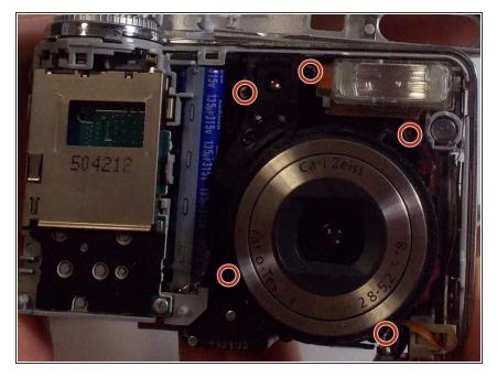
Remove five 2mm Phillips #00 screws surrounding the lens using a screwdriver.
