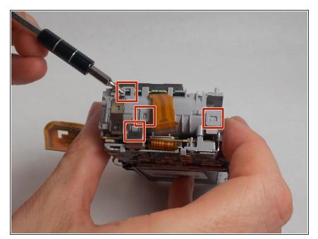
Use a spudger or screwdriver to unhinge the clips. This releases the battery terminal.
