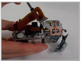
Disconnect the ribbon cables on top of the battery terminal using a spudger or screwdriver.
