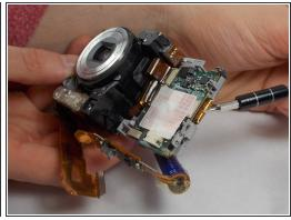
Disconnect the three pictured ribbon cables using a spudger or screwdriver.
