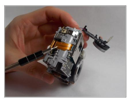
Disconnect the remaining ribbon cable on the side of the camera using a spudger or screwdriver.
