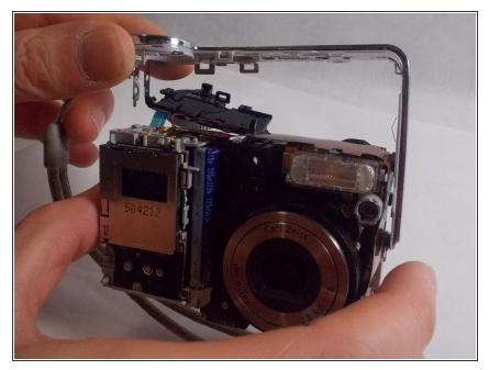
Now the casing can be removed after all latches have been undone.
