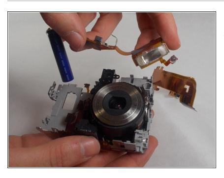
After all clips have been undone the flash is free to be removed/replaced.
