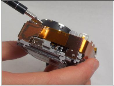
• Release the clips on either side of the connector/ribbon cable using a spudger or screwdriver.
