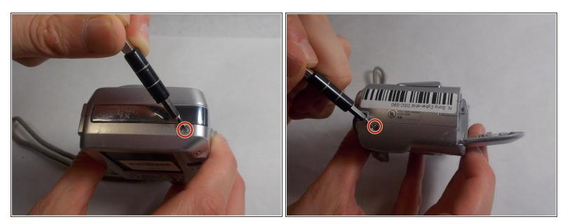
Remove the two 2mm Phillips #00 screws (one on each side of the camera).
