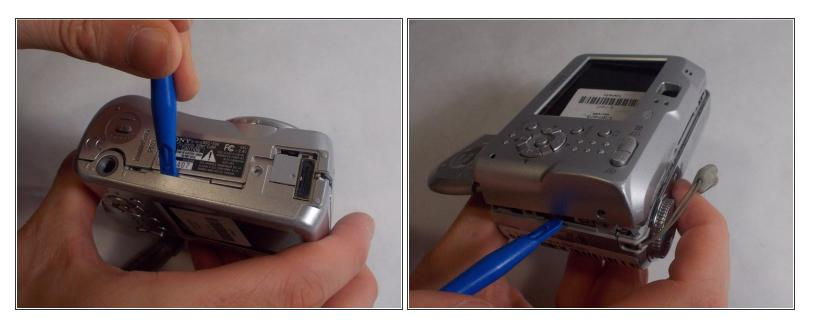
• Use an opening tool to unlock the front case from the main body of the camera. Use the tool on the right side and bottom of the camera with the LCD screen facing you.
