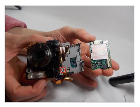
Push the clip to the left and lift the motherboard upwards and away from the camera.
