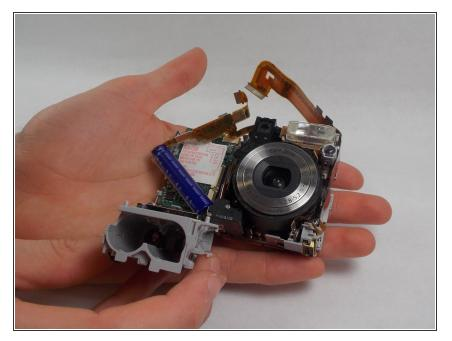
Now the battery terminal can be separated from the main body of the camera.
