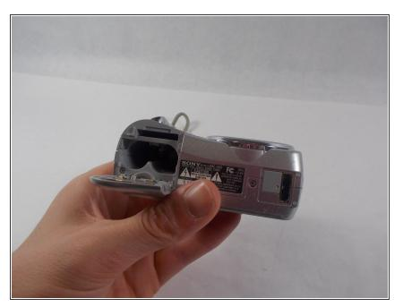
• Pull open the door and allow the batteries to fall out.
