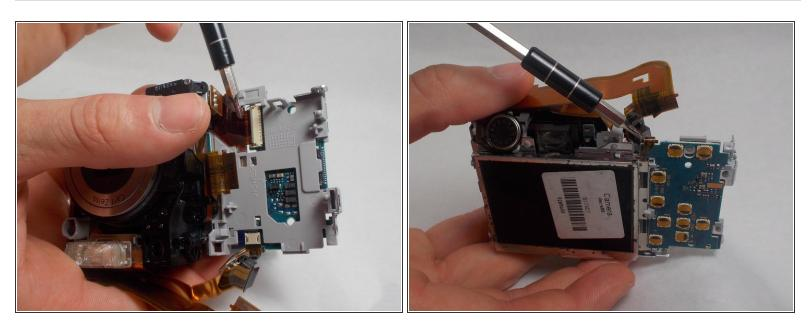
• Disconnect the two ribbon cables using a spudger or screwdriver.
