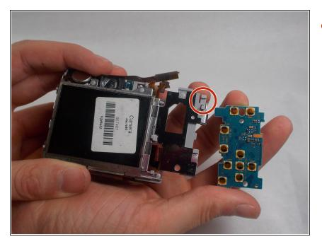
Unlatch the clip and lift the motherboard upwards and away from the camera.
