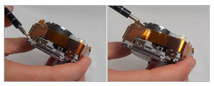
• Release the clips on either side of the connector/ribbon cable using a spudger or screwdriver.
