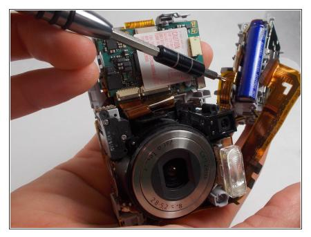
Once the battery terminal is unclipped, pull this ribbon cable out with a spudger or screwdriver to finish freeing the battery terminal.
