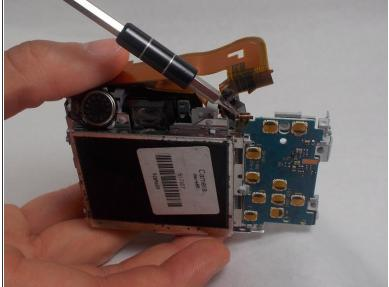
Disconnect the two ribbon cables using a spudger or screwdriver.
