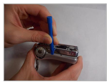
Use an opening tool to unlock the front case from the main body of the camera. Use the tool on the top of the camera.
