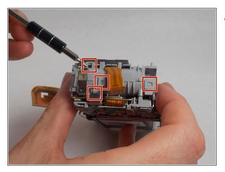
Use a spudger or screwdriver to unhinge the clips. This releases the battery terminal.
