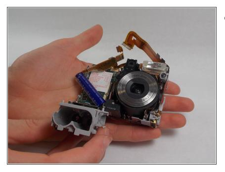
Now the battery terminal can be separated from the main body of the camera.
