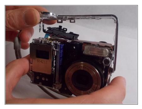
• Now the casing can be removed after all latches have been undone.
