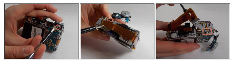
Disconnect the ribbon cables on top of the battery terminal using a spudger or screwdriver.
