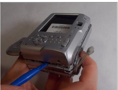
Use an opening tool to unlock the front case from the main body of the camera. Use the tool on the right side and bottom of the camera with the LCD screen facing you.
