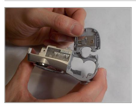
After the front casing is removed, the battery door hinges off freely.
