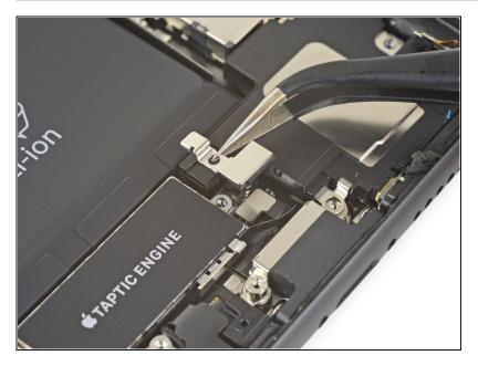
Remove the Taptic Engine connector cover.
