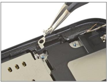
• Remove the small grounding clip on the top right corner of the speaker.
