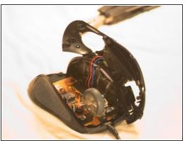
Grab the top shell of the mouse and lift up to remove.
