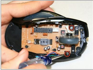
Locate the 5 mm silver flat head mounting screws (2) to the left and right of the scroll wheel and remove with the Phillips #1 screwdriver.
