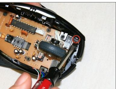
Locate the snaps on the bottom corners of the mouse side panels and pop the indicated snaps out, using a spudger or your fingernail.
