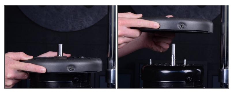
• Lift the blower plate up and remove it from the motor assembly.
