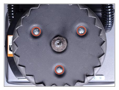
Remove the three 7/16" (11 MM OK) nuts securing the blower plate.
