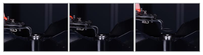
• Use snap ring pliers to remove the retaining ring on the top of the fan axle.
