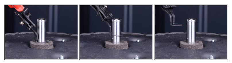
• Use snap ring pliers to pry open and remove the retaining clip at the base of the fan axle.
