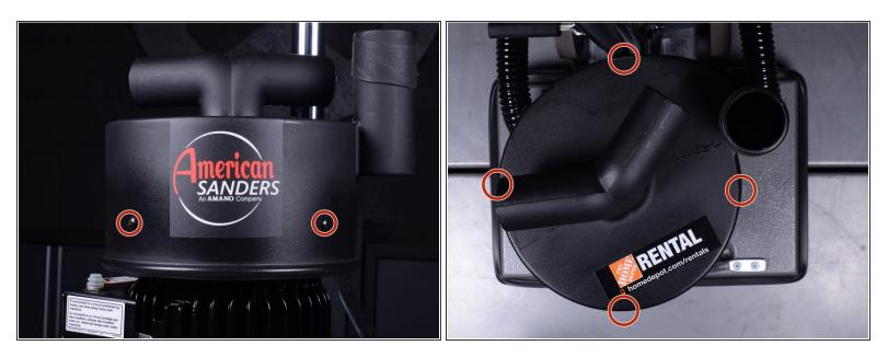
• Remove the four 22mm long Phillips screws around the side of the blower housing.
