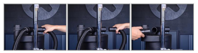
• Twist and pull to disconnect both suction hoses from the blower housing.
