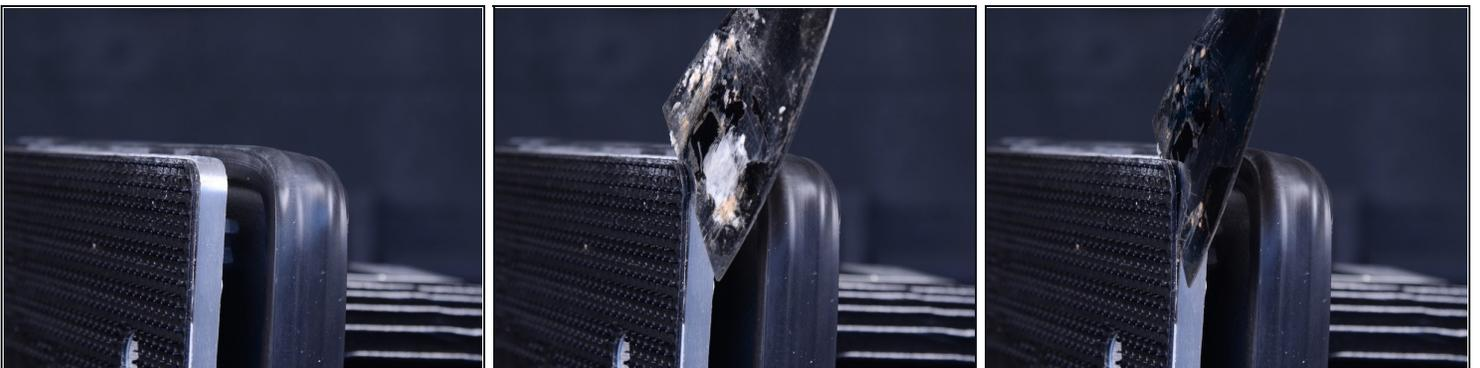
ⓘ The grip face pad is attached to the base plate by a layer of spongy adhesive.
