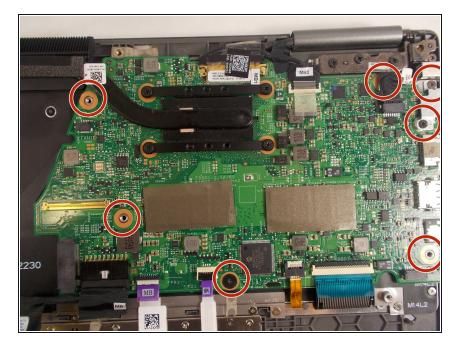
• Remove the seven 2mm screws securing the motherboard.
