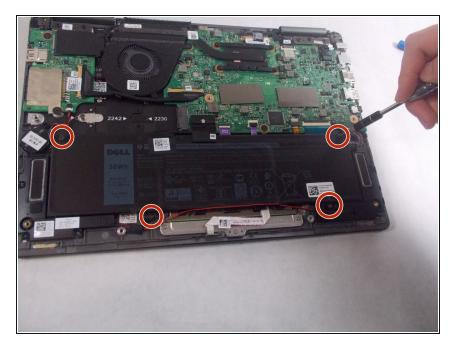
Use a Phillips screwdriver to remove the four screws holding the battery in place.
