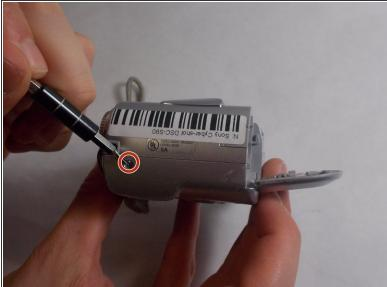
Remove the two 2mm Phillips #00 screws (one on each side of the camera).
