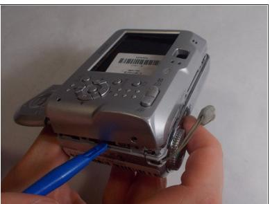
Use an opening tool to unlock the front case from the main body of the camera. Use the tool on the right side and bottom of the camera with the LCD screen facing you.
