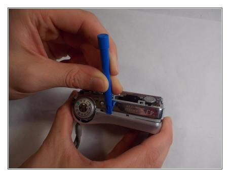
Use an opening tool to unlock the front case from the main body of the camera. Use the tool on the top of the camera.
