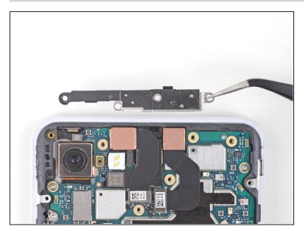
Remove the front camera bracket.
