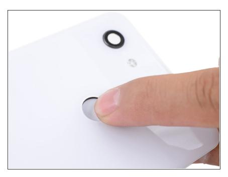
From the outer side of the back cover, use your finger to push the fingerprint sensor out of its cutout.
