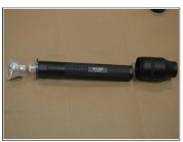
Slide the lens housing down, toward the base, to remove
