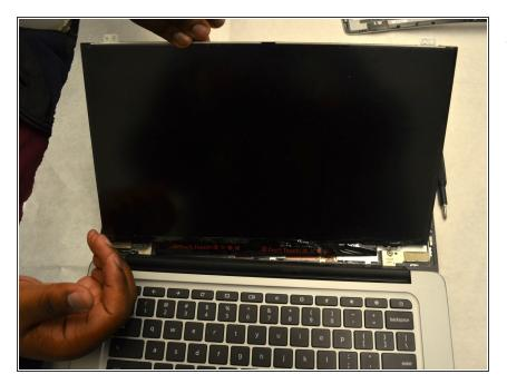
• Pull the screen down, and lay it flat against the keyboard.
