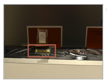
• Disconnect the input connector from the screen.
