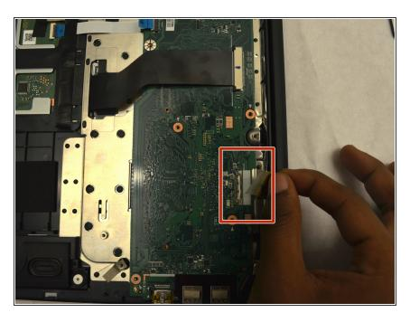
Disconnect the LCD cable from the motherboard by removing the tape on the LCD connector, then gently pulling out the ribbon cable.
