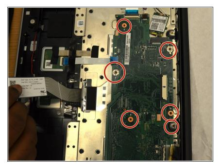
Remove the seven 4mm JIS #0 screws that hold the motherboard in place.
