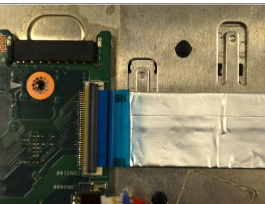
Disconnect the daughterboard from the motherboard by gently removing the daughterboard cable from the motherboard connector.
