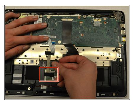
Disconnect the trackpad by pulling on the trackpad connector cable.
