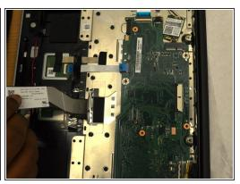
Disconnect the LCD cable from the motherboard by gently pulling on the cable.
