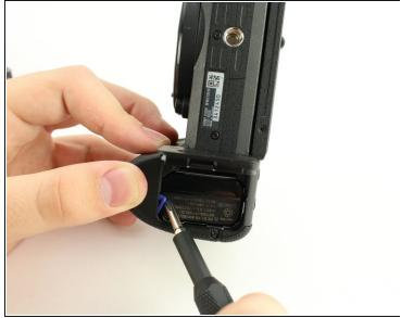
Push the blue lever aside to release the battery.
