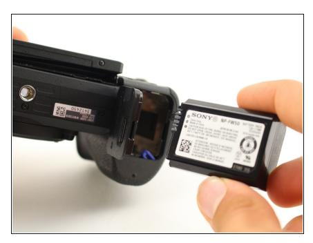
Remove the released battery from the compartment.
