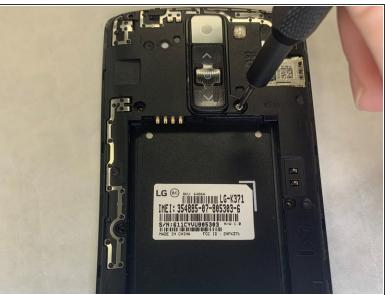
Remove all nine of the 3.0mm screws on the back of the phone using a Phillips #0 screwdriver, including the one attaching the camera lens.
