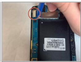
• With a plastic opening tool, disconnect all three ribbon connectors from the motherboard: one for the front camera, one for the rear camera, and one for the screen.
