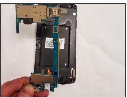
Using a plastic opening tool, separate the motherboard from the back frame and remove it from the device.
