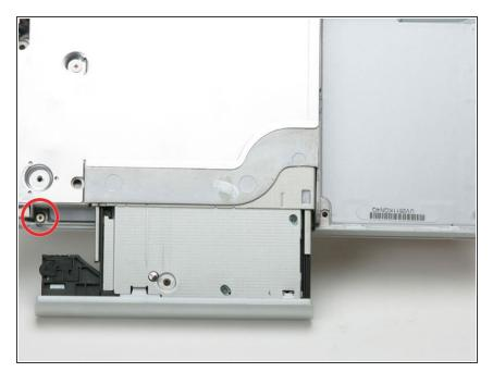
Pull the optical drive a bit more so that you can access and remove a second Phillips screw near the power receptacle.
