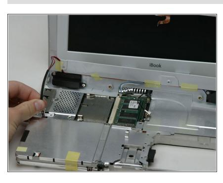
Lift the upper case off completely and disconnect the red and black speaker cable from the logic board.
