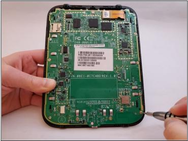
① Use an anti-static mat to prevent electric shock from damaging the motherboard and its components. Be careful when using metal tools on your device.
