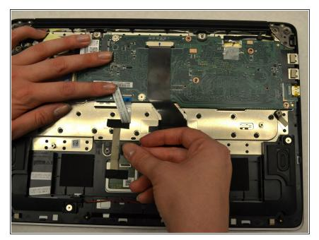
• Unclip the motherboard connector from the track pad.
