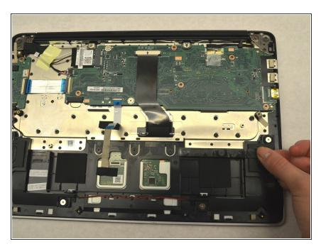
• Remove the strip of electrical tape from across the top of the track pad.
