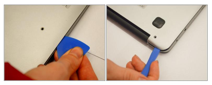
Insert an opening pick between the back panel and the sides of the computer to begin lifting the back off.
