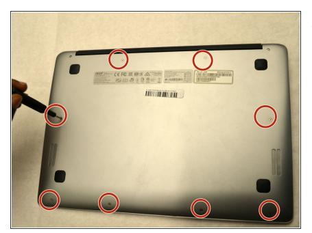
Remove the eight 4mm JIS #0 screws from the back cover.
