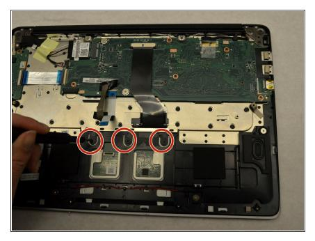
• Remove three 4 mm JIS #0 screws from the top of the track pad.
