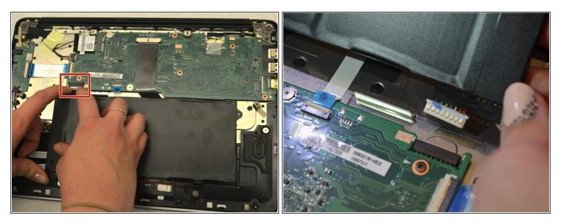
• Pull the white tab connected to the battery out of the black tab that connects to the motherboard.
