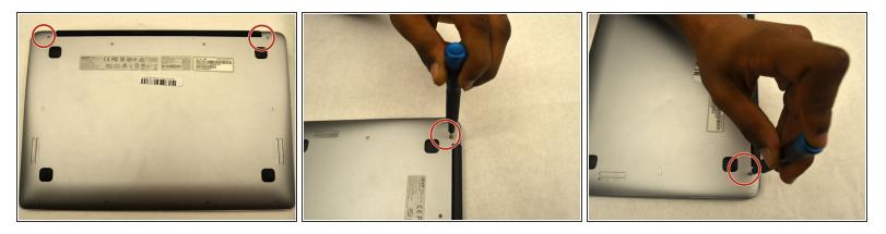
Remove the two 6mm JIS #0 screws from either side of the hinges.
