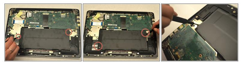
Remove the two JIS #0 screws that connect the battery to the rest of the laptop.
