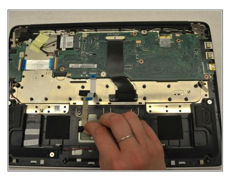
Remove the strip of tape that secures the motherboard connector to the track pad.
