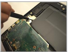
Remove the two JIS #0 screws that connect the battery to the rest of the laptop.
