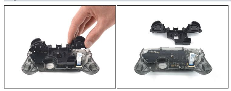
Remove the trigger buttons from the plastic cover.
