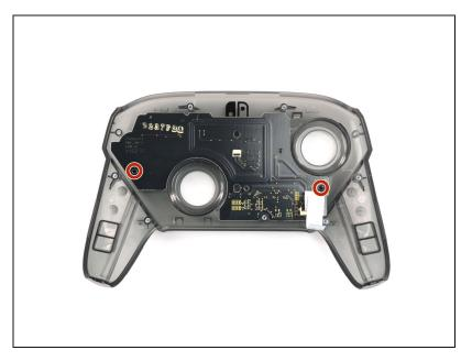
Use a Phillips screwdriver to remove the two 5 mm-long screw securing the circuit board.
