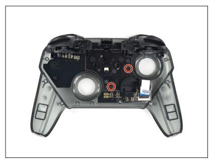
Remove the two 6.8 mm-long screws on the top circuit board using a Phillips screwdriver.
