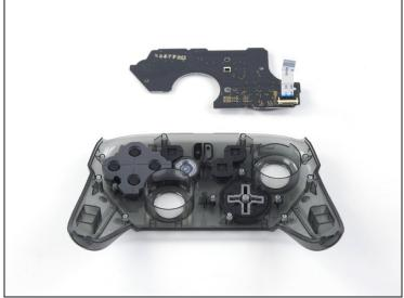
• Remove the circuit board.
