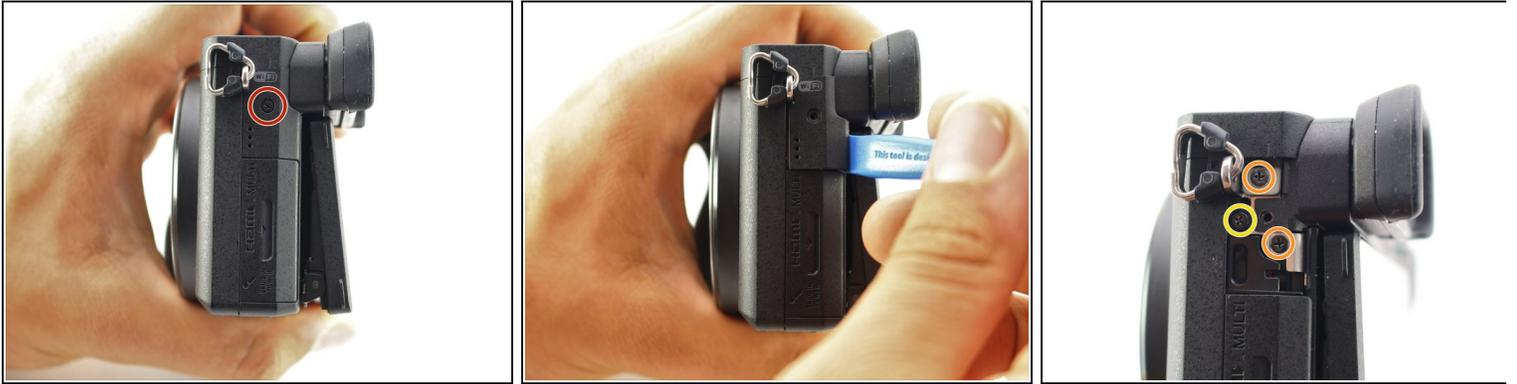
**i** To remove the top of the camera you must remove the back first.
