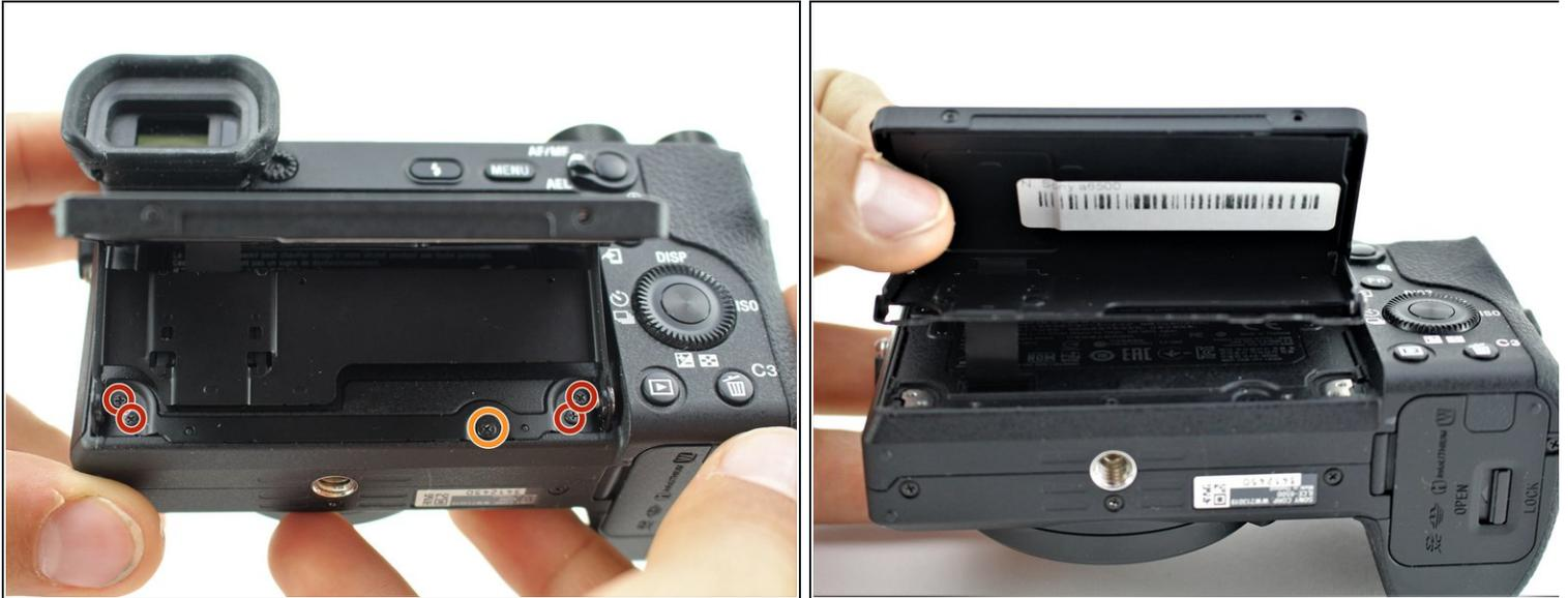
**i** To access the back of the camera remove the screws attaching the LCD screen hinge to the camera body.
