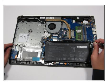
Remove the screws holding the battery in place using a Phillips #1 screwdriver.
