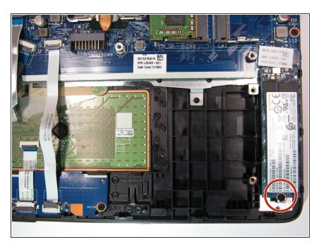
Remove the screw holding the SSD in place using the Phillips #1 screwdriver.
