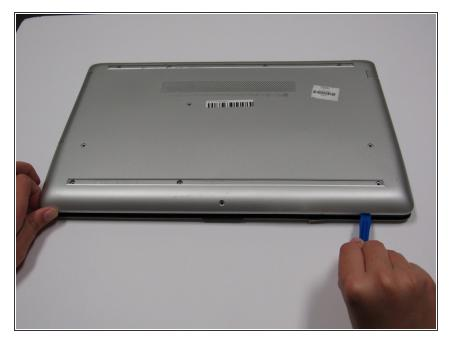
Close the screen and flip over the laptop. Using the plastic opening tools, gently take off the back cover starting from the middle, bottom edge.
