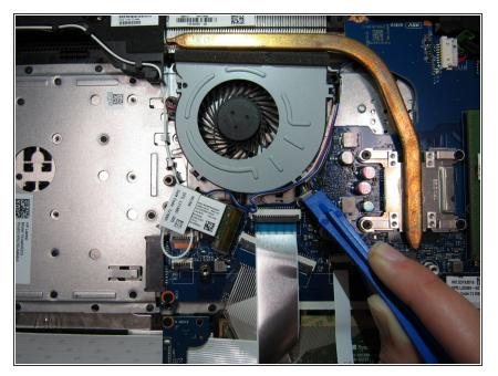
Pull out the connector for the fan cable using the opening tool or spudger.
