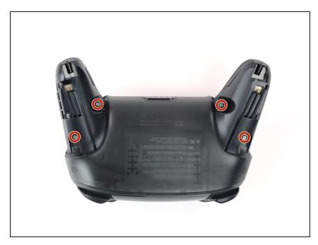
Use a JIS #00 screwdriver to remove the four silver 6.8 mm screws that secure the clear back plastic cover.
