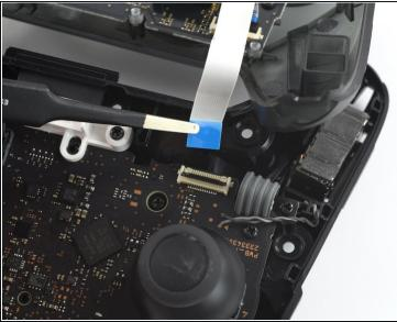
• Use your fingers or a pair of blunt nose tweezers to disconnect the interconnect cable from its connector.
