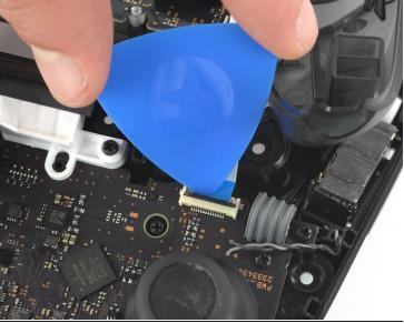
Use the tip of an opening pick to open the black flap of the ZIF connector by pushing it upwards.
