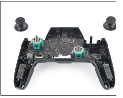
• With light force pull the two joystick caps off of the controller.
