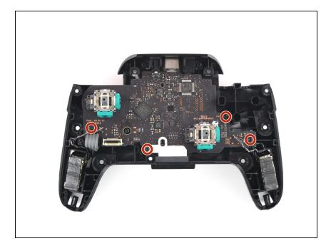
Use a Philipps screwdriver to remove the four 5 mm-long screws securing the motherboard.
