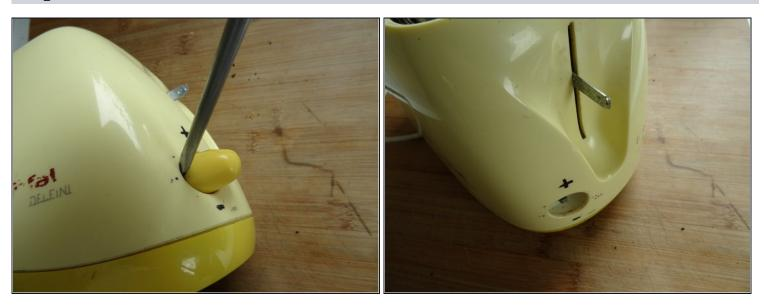
• Also pull off the knob on the controller, a lever tool was used here.
