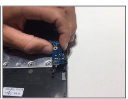
• Carefully remove the aux port from the frame of the computer as shown.
