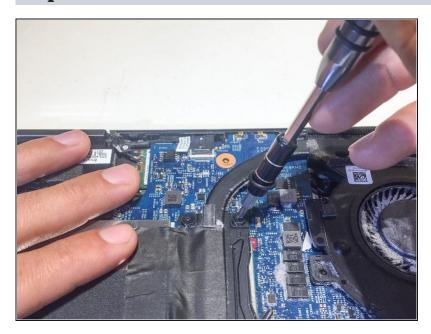
Remove the four spring loaded screws with a Philips #1 screwdriver.
