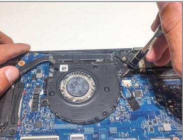
• Using a Philips #0 screwdriver, remove the three M2x4 screws located around the cooling fan as shown in this picture.
