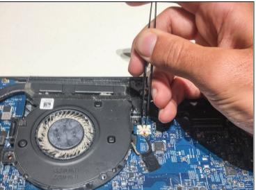
• Remove the connector clip with the tweezers.
