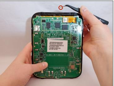
Use tweezers to remove the brass-colored threaded fastener from the Nook plastic casing.
