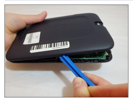
Slide the back cover down towards the USB port to release it. The pictures show the case being prised open but this should not be necessary.
