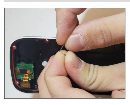
Strip the ends of the red and silver wires connected to the back panel of the device using a pair of wire strippers.
