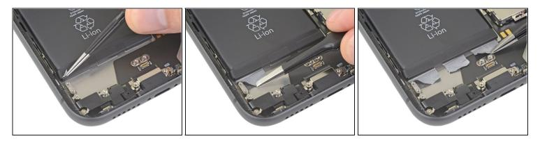
Peel back the three battery adhesive pull tabs from the bottom edge of the battery.
