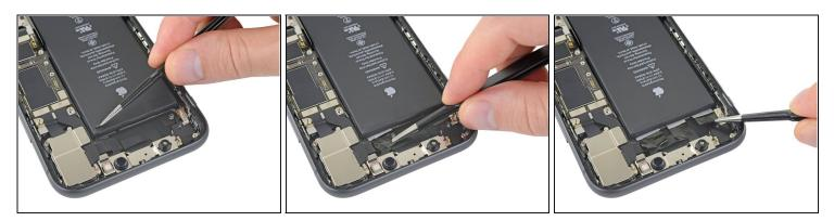
Peel back the three battery adhesive tabs from the top edge of the battery.
