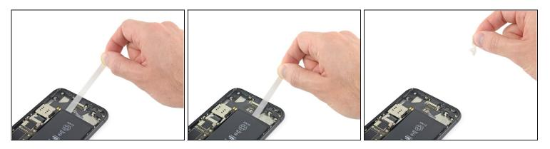
• Repeat the above steps to remove the other two adhesive strips near the bottom edge of the iPhone.
