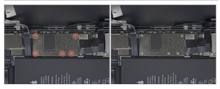
• Use a Y000 driver to remove the five 1.1 mm screws securing the logic board cover bracket.
