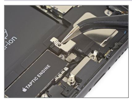
• Remove the Taptic Engine connector cover.
