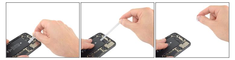
• Pull the top adhesive strips out one at a time, using the same method you've used to pull the bottom strips.
