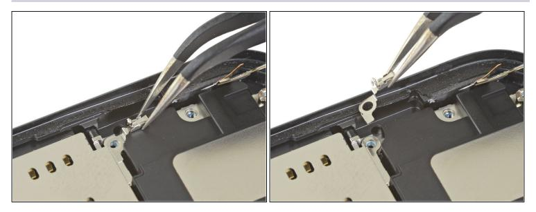
• Remove the small grounding clip on the top right corner of the speaker.
