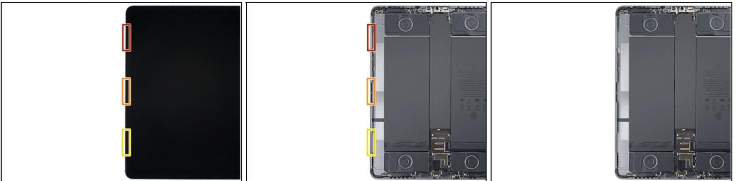
⚠ There are three cutouts along the left edge of the screen where the adhesive is very thin. Don't insert your opening pick more than **2 mm** to avoid damaging the screen at these cutouts:
