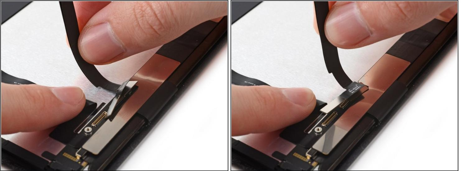
**i** The display cable is lightly adhered to the screen.
