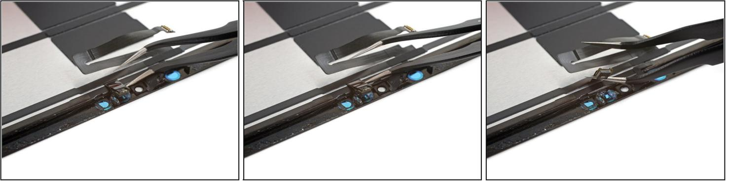
**⚠** Be very careful during this step, as the sensor cable can tear. Work slowly and apply more heat if you encounter resistance.
