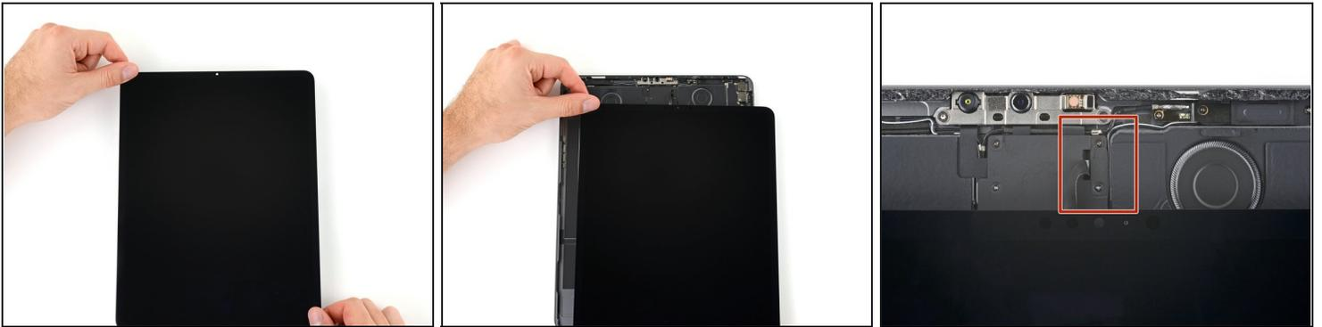
**⚠ Don't fully remove the screen, as it's attached to the frame by several cables.**
