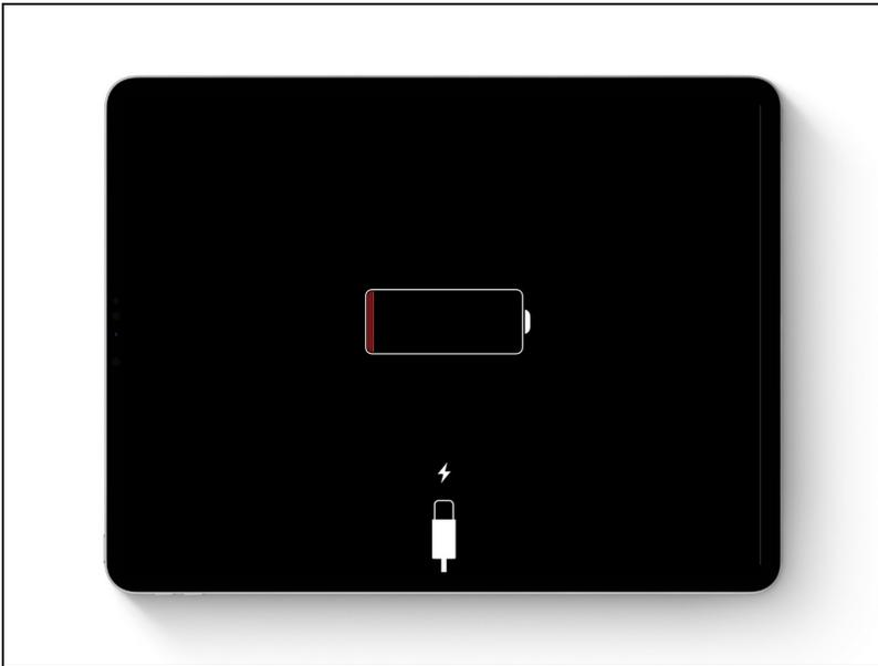
⚠ Allow your iPad's battery to fully drain before starting this repair. A charged battery may catch fire if damaged during the repair.
