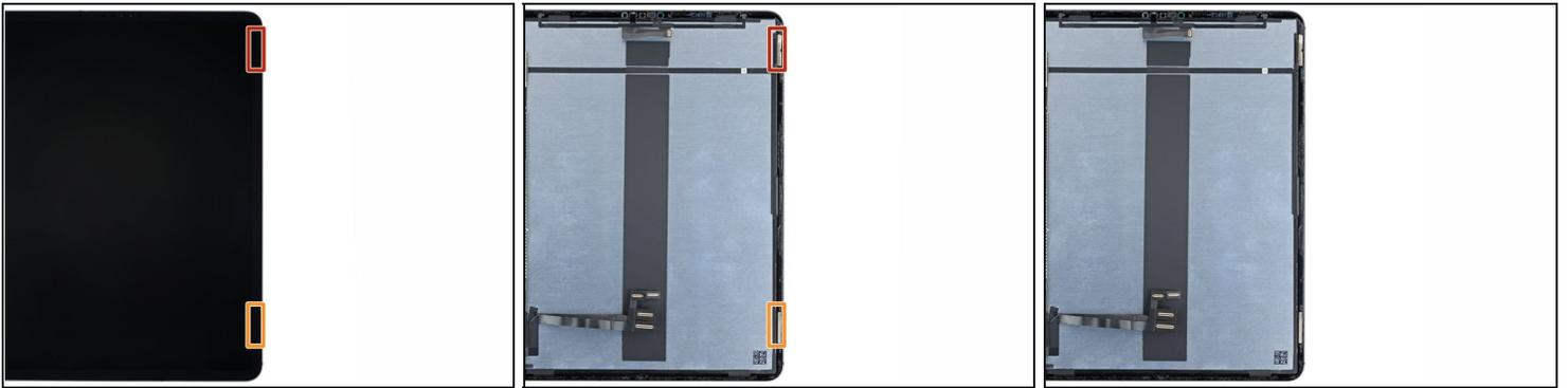
⚠ There are two **2 cm-long** magnets along the right edge of the screen. Don't insert your opening pick more than **2 mm** to avoid damaging the screen in these locations:
