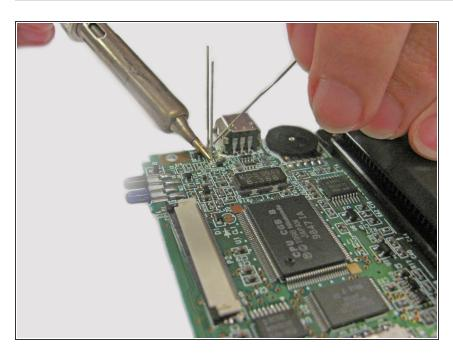
Solder the leads of the new LED to the circuit board.
