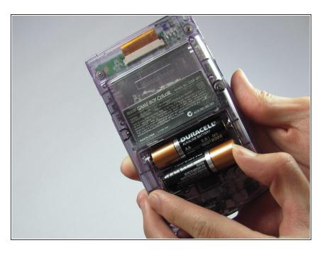
Remove the batteries from the battery compartment.
