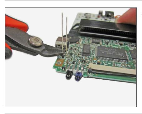
Cut the excess ends of the LED legs using the wire cutters.
