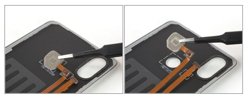
• Remove the fingerprint sensor.
