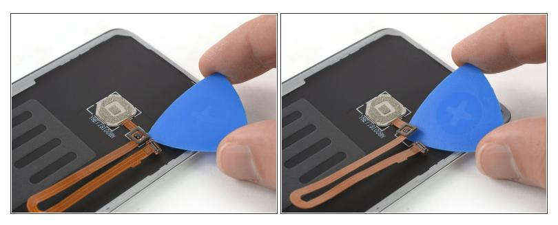
• The fingerprint flex cable is mildly glued to the rear glass. Carefully slide an opening pick underneath to separate it from the glass.
