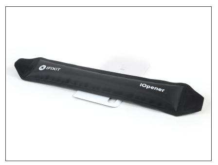
Apply a <u>heated iOpener</u> to the rear glass to loosen the adhesive beneath the fingerprint sensor. Apply the iOpener for at least two minutes.
