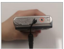
• Remove all seven 3mm screws by using the Phillips #1 screwdriver.
