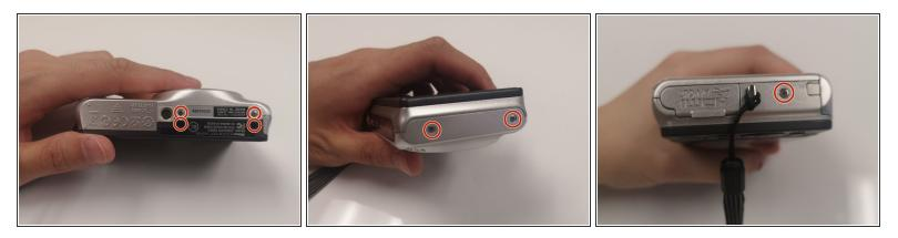
Remove all seven 3mm screws by using the Phillips #1 screwdriver.
