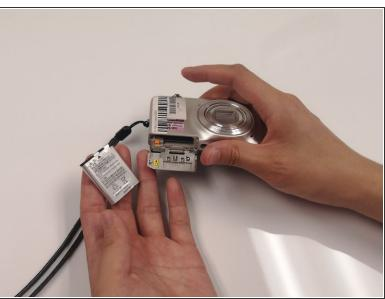
Remove the battery by pushing the orange flap down. Replace the battery with the new one.
