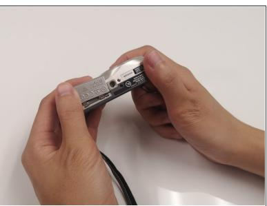
Open the battery door by keeping the display screen in your direction. Apply pressure on the door and press and slide it forward.
