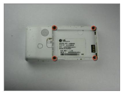
Use a Phillips #00 screwdriver to unscrew the four Phillips #00 screws on the four corners under the battery to unfasten the back case from the phone.
