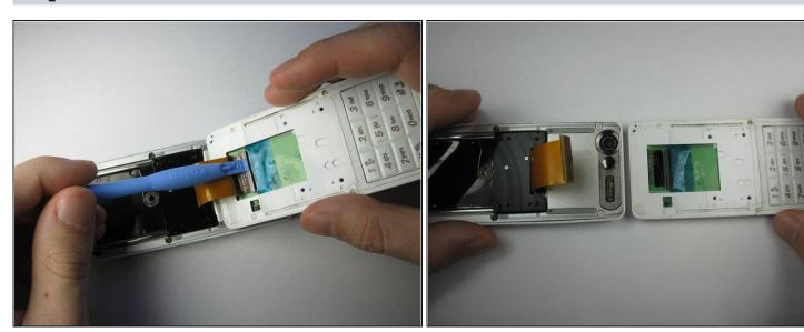
Between the two halves is a ribbon. Use a plastic opening tool to flip up the lock and disconnect it.
