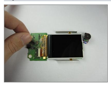
Next, carefully remove the tape from the LCD board.
