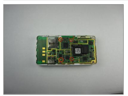
Unscrew the 4 Phillips 00 screws that connect the two halves of the phone together.
