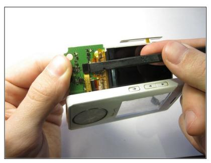
• Unhook the ribbon cable using that flat side of a spudger.
