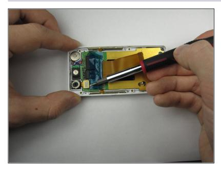
Carefully pry the connecting cable between the camera and the motherboard off of the board.
