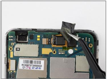
• Carefully remove the protective sticker. This will expose the camera and its connector.
