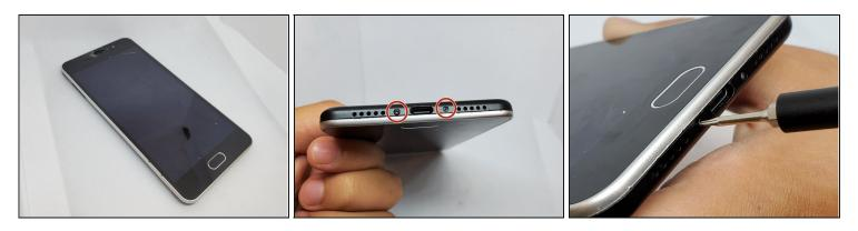
Remove two 2mm TR9 Torx screws from the bottoms of the device.
