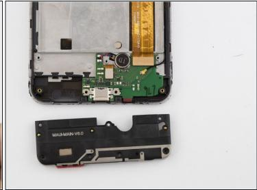
Use a pair of angled tweezers to remove the speaker housing.
