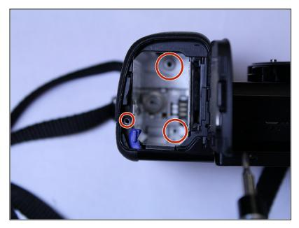
Once the battery is removed, use a Phillips #00 screwdriver to remove the three screws at the bottom of the battery compartment.
