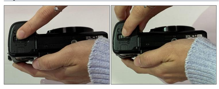
• Slide the notched locking bar on the battery compartment from LOCK to OPEN.
