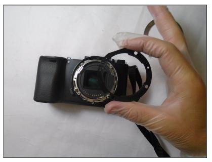
• Carefully remove the black ring from the lens assembly.
