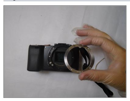
Carefully remove the outer most silver ring from the lens assembly.
