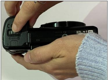
Slide the notched locking bar on the battery compartment from LOCK to OPEN.
