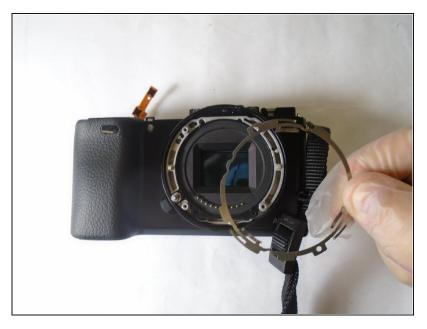
Carefully remove the thin silver ring from the lens assembly.
