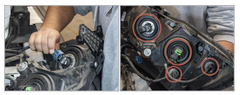
Press the tab on the connector and pull. Do this for all 4 connectors.
