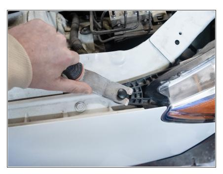
• Use the clip remover tool to pry the clip up to remove it.
