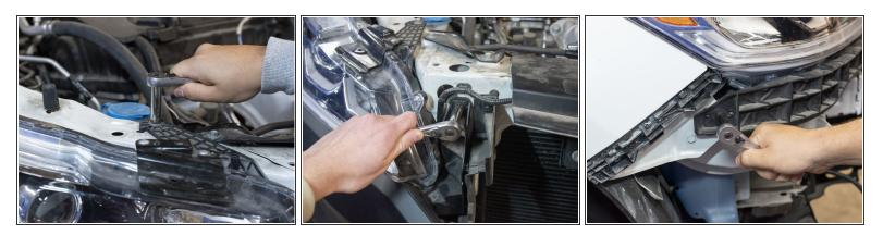
• Use a 1/4" ratcheting wrench and a 10mm socket to remove the three bolts.
