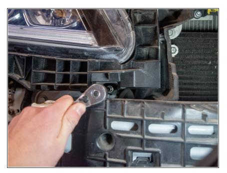
Use a 1/4" ratcheting wrench, a 6" extension and a 10mm socket to remove the last bolt.
