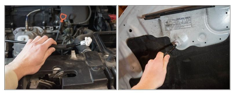
• Lift up the hood prop rod and insert it into the hole on the underside of the hood.
