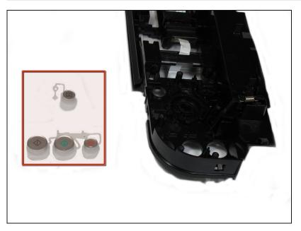
Remove the buttons from the plastic button assembly.
