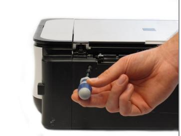
• Remove the two 7.9 mm screws using a Phillips #1 screwdriver.
