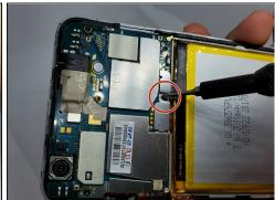
⚠ Before continuing, tighten the <u>anti-static wrist strap</u> around your wrist and connect the alligator clips to a metal portion of the phone.
