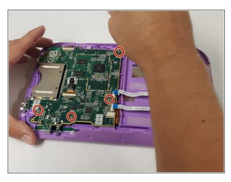
Unscrew the four 5.0 mm Phillips #0 screws securing the motherboard.
