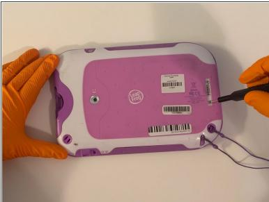
Remove the two 5.0mm Phillips #0 screws.
